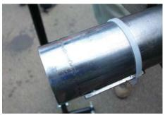
While on the topic of kart rear axles, the image shows an example that was rejected at scrutineering due to the fact that it has an additional section welded on to the end. Scrutineers have been instructed to ask competitors to change any axles that have been modified in such a way as to contravene the regulations.
